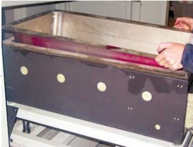
Figure 2. Titanium solder pot liner prevents iron dissolution and increases the life of the solder pot.
